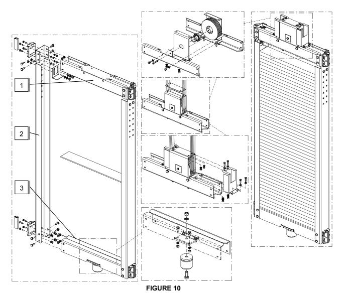
The counterweight frame is consisted of three main parts:
