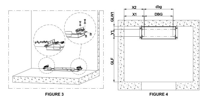
Firstly, locate the two plates for the main and auxiliary guide rails to the pit floor as shown in FIGURE 3. Their exact location according to shaft walls is determined after the guide rails are placed as shown in FIGURE 4.
