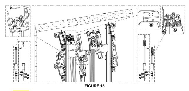
Caution: The spring on the wedge sockets are placed only at the side of the counterweight frame.
